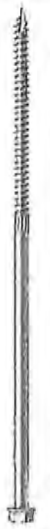
1/2" X 8" SCREW #D5025800 USED TO SECURE 4" X 4" ANGLE BRACES AT TWO 10" X 10" POSTS. SEE SECTION B-B ON SHEET NO. 4 AND DETAIL NO. 3 ON SHEET NO. 5
