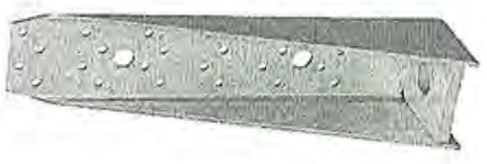
HOLDOWN #HHDQ11-SD52LS USED ON 10"X10" POSTS. 2/PER POST. USE 1" WEDGE ANCHORS AT BASE AND 1/4"X2 1/2" SD5 SCREWS ON TOP PORTION. SEE SECTION A-A ON SHEET NO. 4
