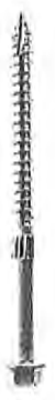
1/2" X 2 1/2" SCREW #D5052511Z USED ON TOP PORTION OF HOLDOWN SHOWN ABOVE. ALSO USED ON 2" X 4" 138" BACKER USED TO SUPPORT 45 DEGREE ANGLE BRACES AT 10" X 10" POSTS. SEE DETAIL NO. 3 ON SHEET NO. 5
