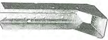
CONCEALED JOIST HANGER #HJ100 FOR 2X10. USE 505 1/2" X 2 1/2" HEAVY DUTY CONNECTOR SCREWS SHOWN BELOW. USED TO CONNECT (2)-2X10'S TO 10X10 POST AT FRONT LEFT LOCATION
