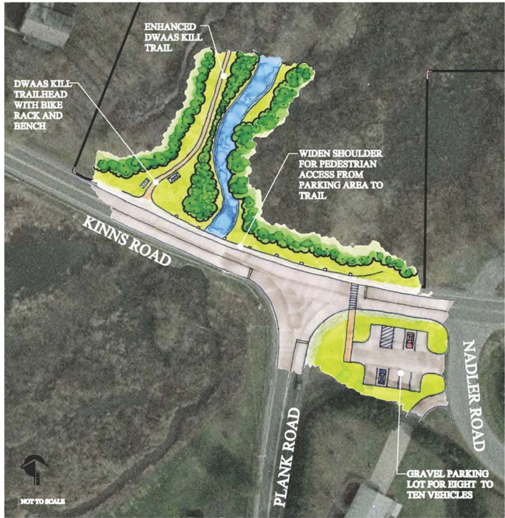
KINNS AND PLANK ROAD INTERSECTION: POSSIBLE PARKING AND ACCESS TO DWAAS KILL TRAIL HEAD ALTERNATE LAYOUT
