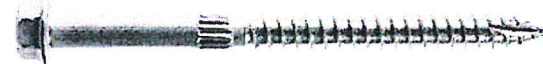
1/4"X2 1/2" SCREW #SDS25212 USED ON TOP PORTION OF HOLDOWN SHOWN ABOVE. ALSO USED ON 2" X 4"X 18" BACKER USED TO SUPPORT 45 DEGREE ANGLE BRACES AT 10" X 10" POSTS. SEE DETAIL NO. 3 ON SHEET NO. 5
