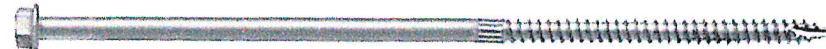
1/4" X 8" SCREW #SDS25800 USED TO SECURE 4" X 4" ANGLE BRACES AT TWO 10" X 10' POSTS. SEE SECTION B-B ON SHEET NO. 4 AND DETAIL NO. 3 ON SHEET NO. 5
